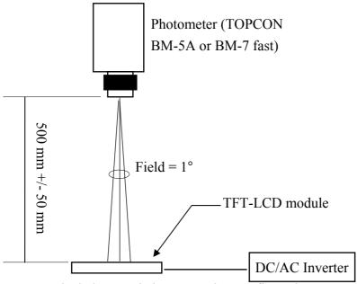
Optical characteristics measuring configuration
