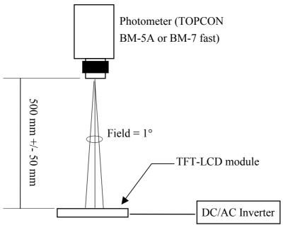
Optical characteristics measuring configuration
