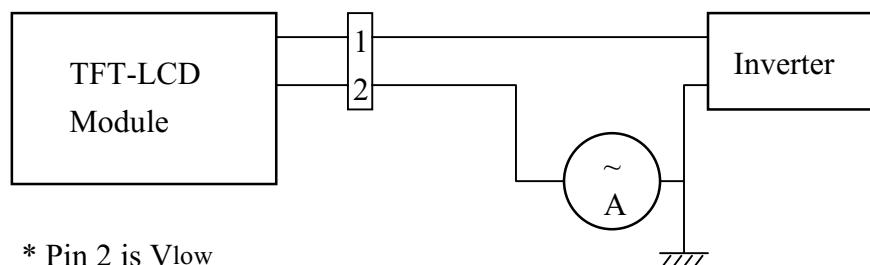
Lamp current dissipation testing configuration
