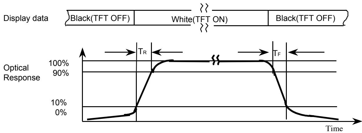
Note 4) After stabilizing and leaving the panel alone at a given temperature for 30 min , the measurement should be executed. Measurement should be executed in a stable, windless, and dark room.
