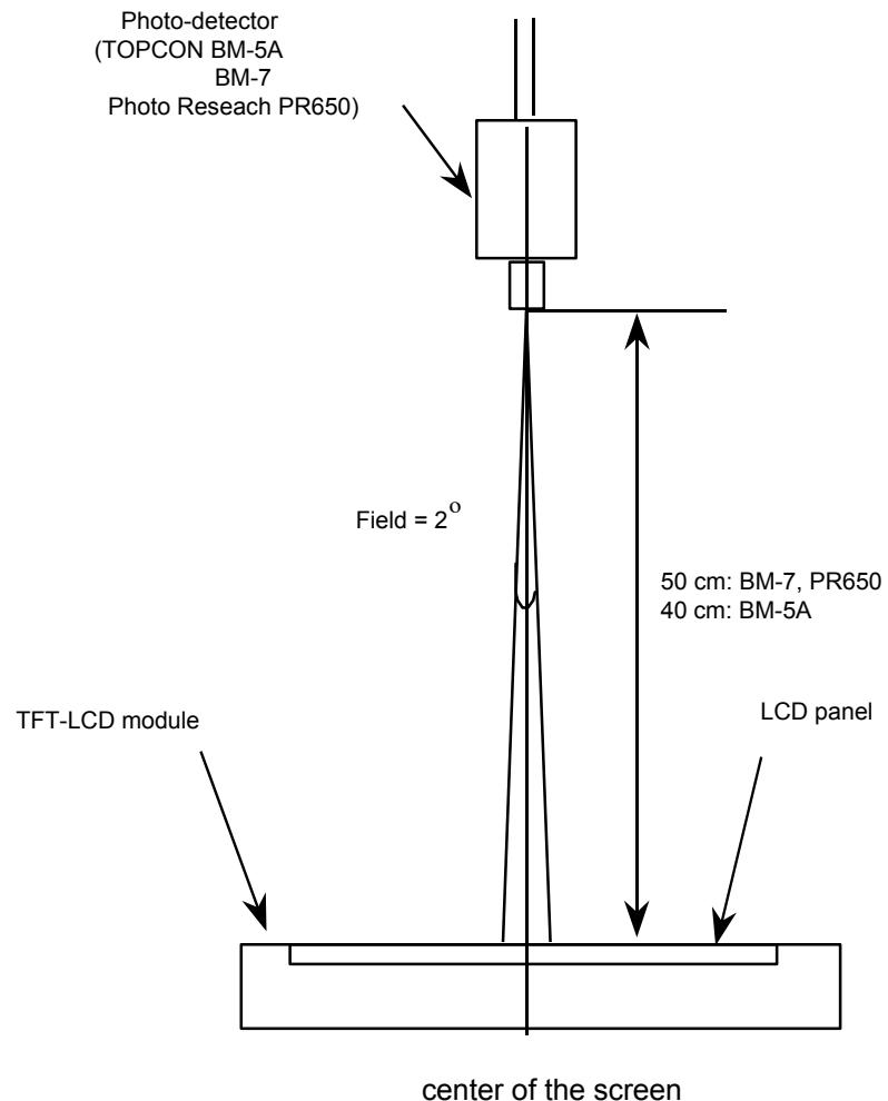
Optical characteristics measurement setup
