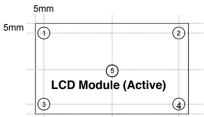
$\Delta T$  should be less than  $10 {}^\circ\text{C}$  ( $\Delta T = |T_{\text{CENTER}} - T_{\text{CORNER}}|$ )
