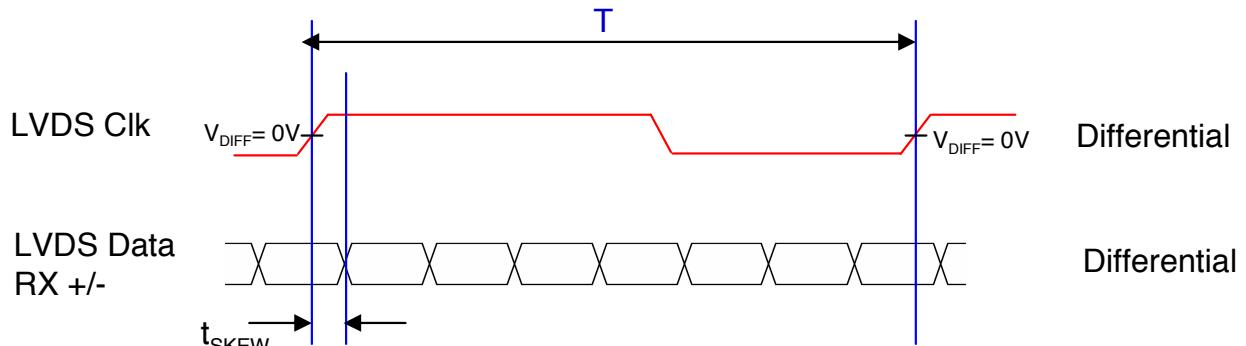
where  $t_{SKEW}$  : skew between LVDS clock & LVDS data,
