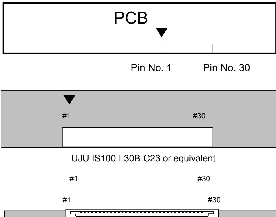
**Fig. Connector diagram**
