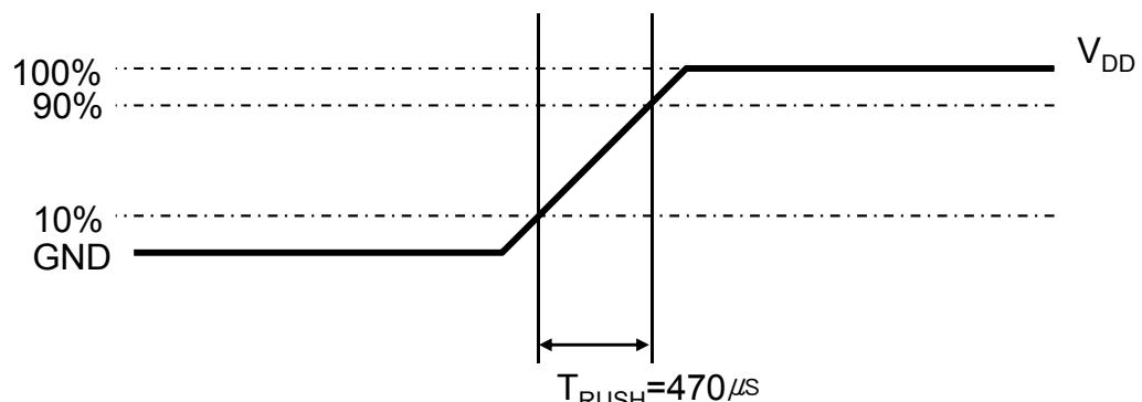
Rush Current  $I_{RUSH}$  can be measured when  $T_{RUSH}$  is  $470\mu s$ .
