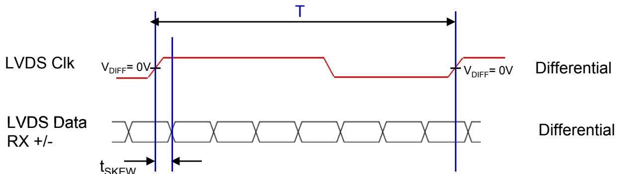
where  $t_{skew}$  : skew between LVDS clock & LVDS data,
