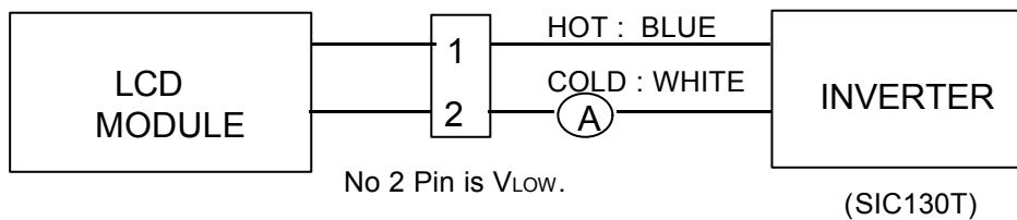
(2) Lamp frequency may produce interference with horizontal synchronous frequency and this may cause line flow on the display. Therefore lamp frequency should be detached from the horizontal synchronous frequency and its harmonics as far as possible in order to avoid interference.
