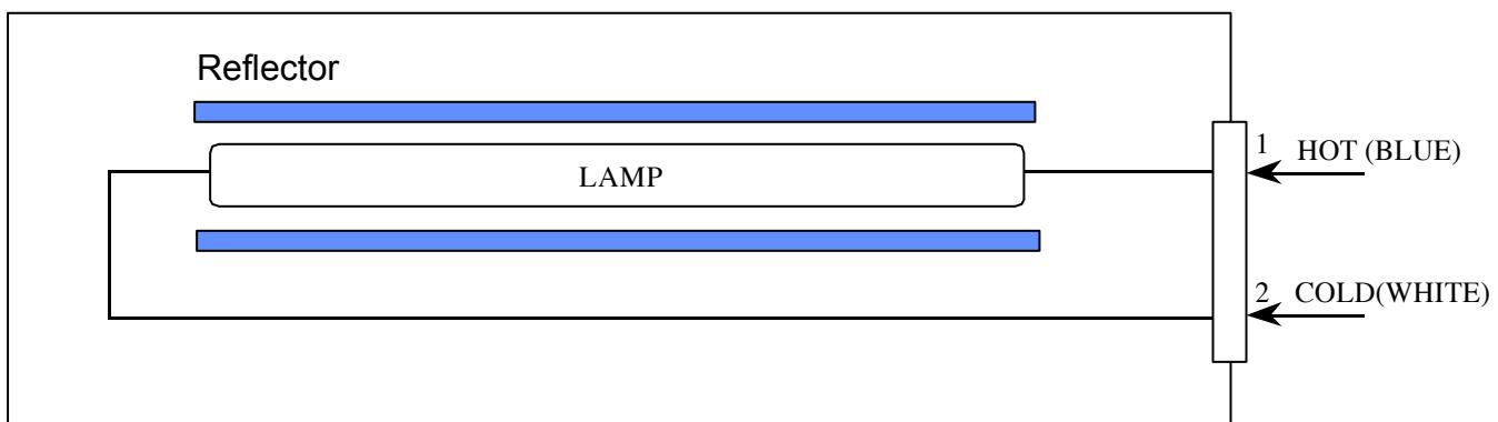
Note) The output of the inverter may change according to the material of the reflector.
