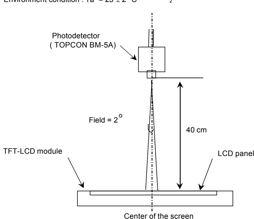
Optical characteristics measurement setup
