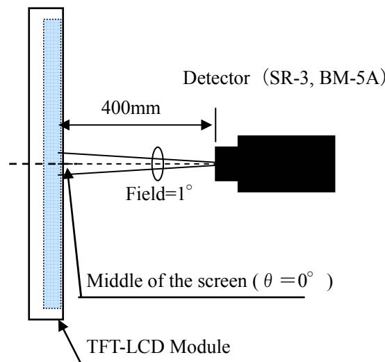
Fig.4-2 Measurement of Contrast, Luminance, Chromaticity and Response time.
