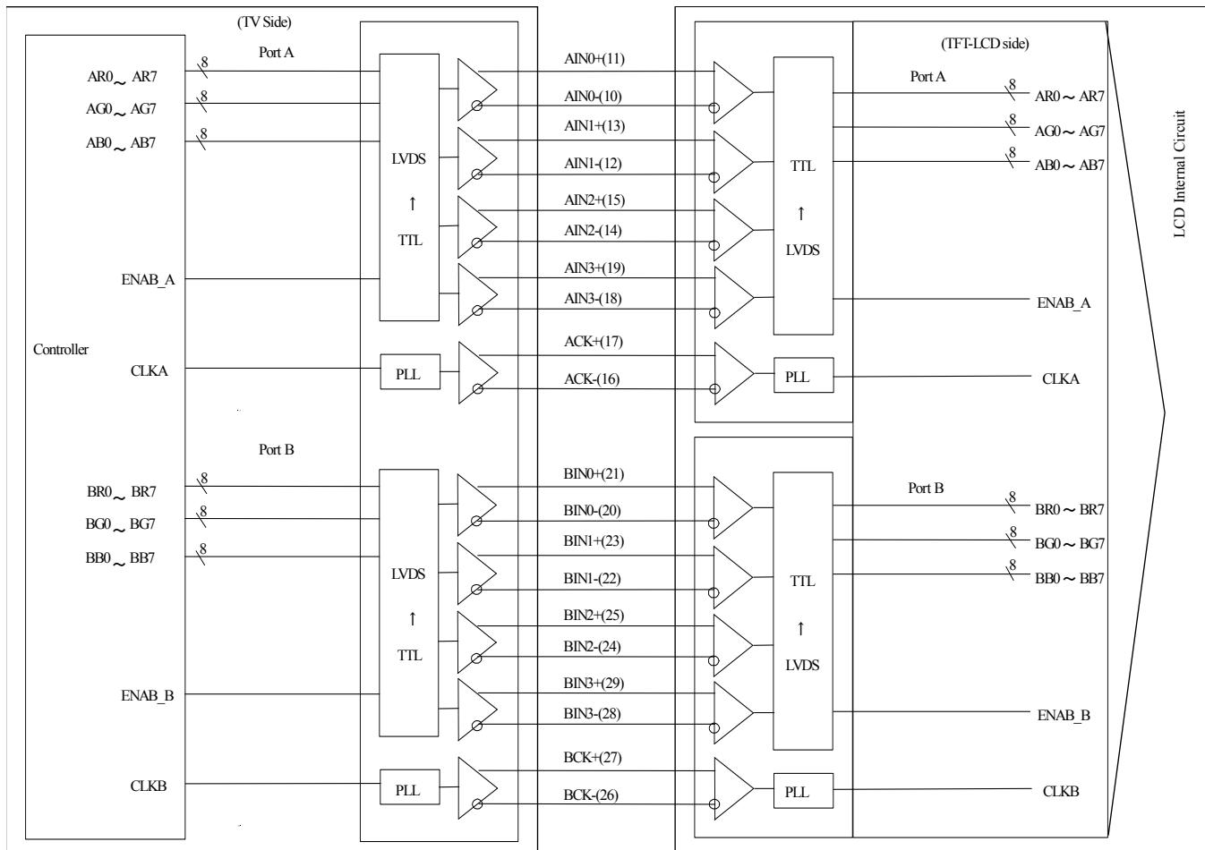
Corresponding Transmitter: THC63LVDM83R (THine) or equivalent device
