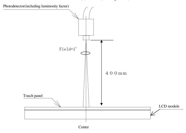
Measuring method (c) for optical characteristics
