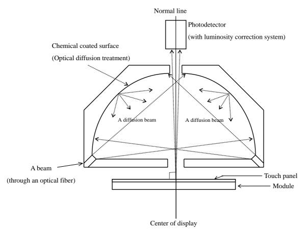
Measuring method (a) for optical characteristics
