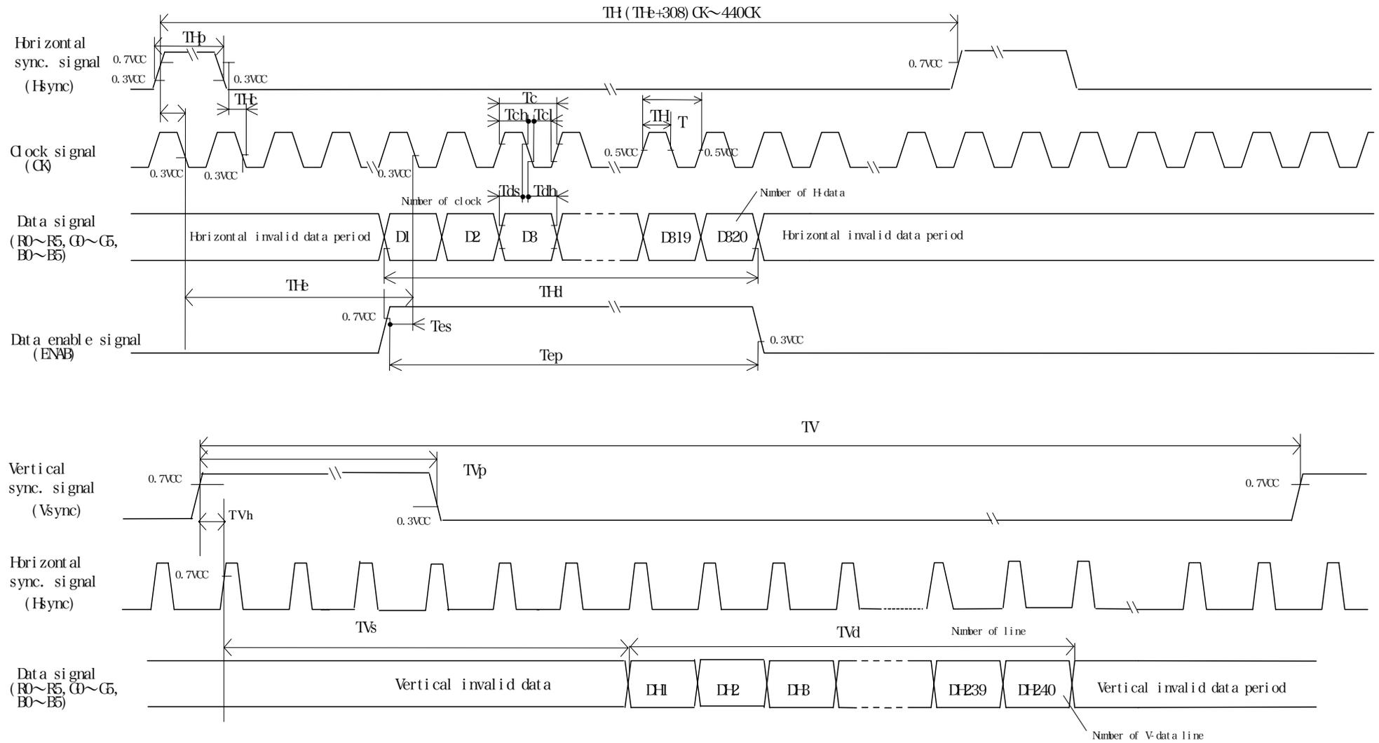
Fig.3-A Input signal waveform
