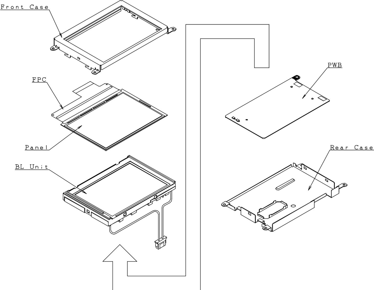
Fig.2. Structure of the module
