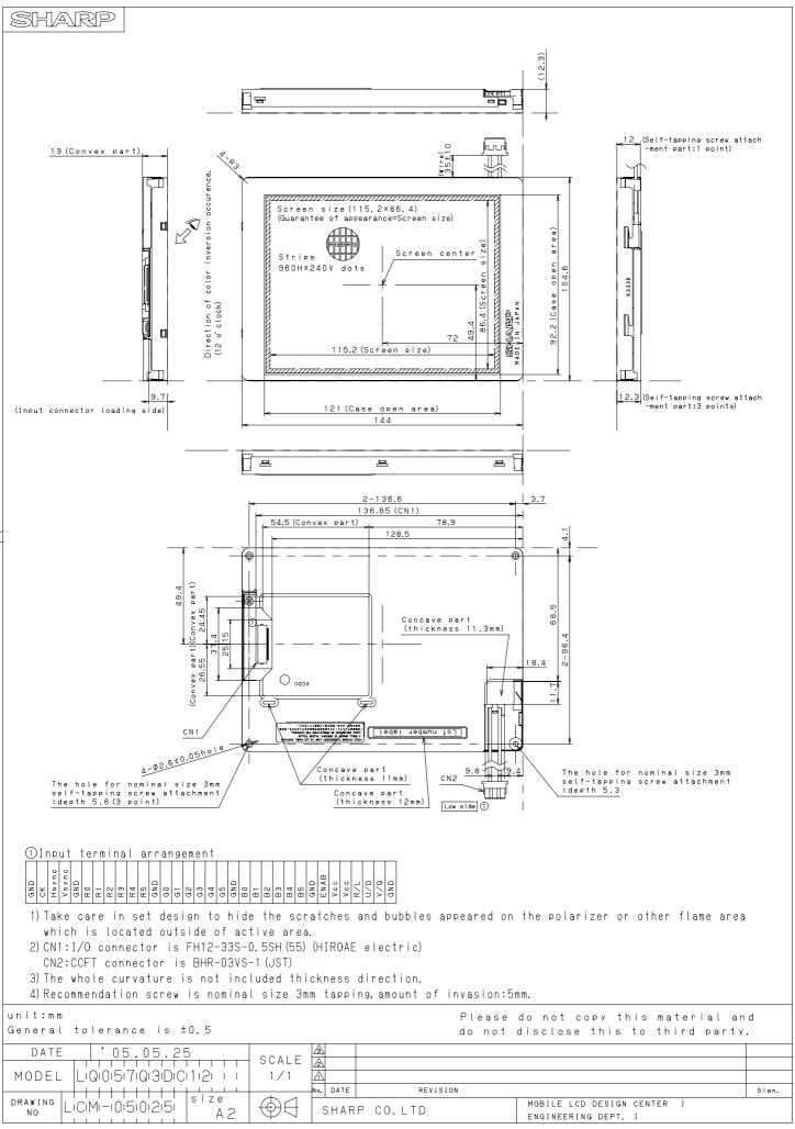
Fig. 1 DIMENSIONS OF THE MODULE
