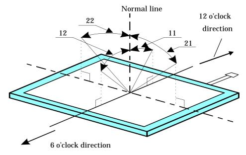
The best viewing angle of this module is slightly leaned to 12 o'clock from normal line. Where  $_{11} > _{max}$ , gray scale is reversed partially. Where  $_{11} < _{max}$ , or in  $_{12}$  direction, gray scale isn't reversed.
