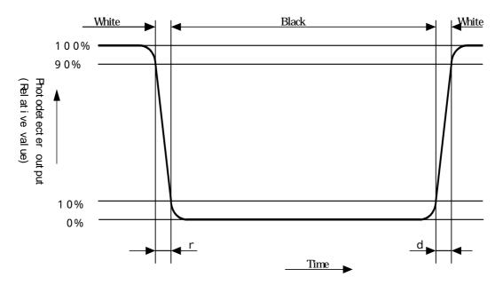
【Note 9-4】 This parameter should be measured at the center of the screen and 30 minutes after turnon. Inverter frequency: 49kHz
