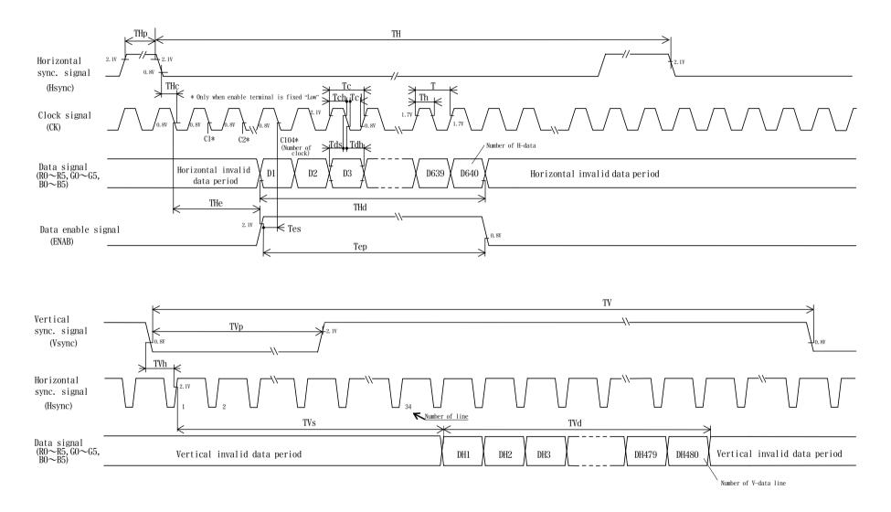
図2-③ Input signal waveforms (350 line mode)
