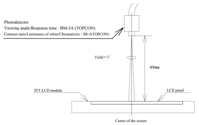
Fig.3 Optical characteristics measurement method
