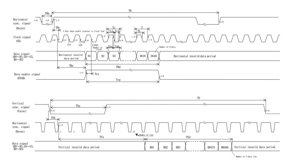
図2-① Input signal waveforms (480 line mode)
