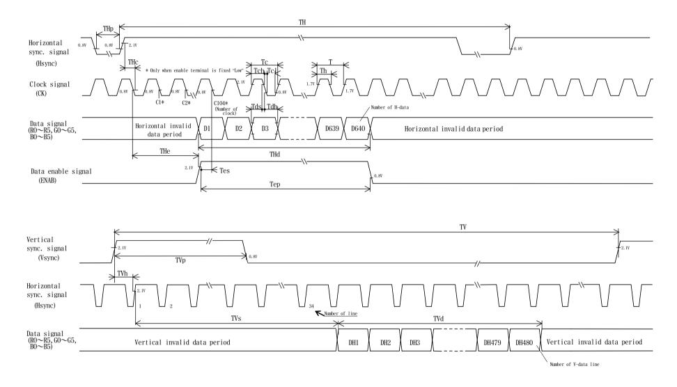
図2-② Input signal waveforms (400 line mode)
