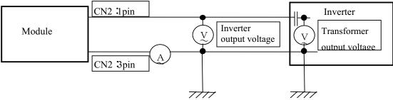
[Note2] Referential data per one CCFT by calculation. (I L  $\times$  VL) The data don't include loss at inverter. (IL=6.0mArms)
