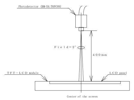
Fig. 3 Optical characteristics measurement method
