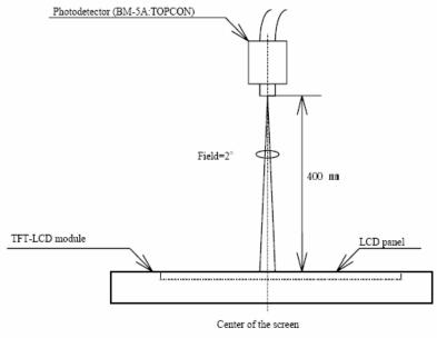
Fig.3 Optical characteristics measurement method
