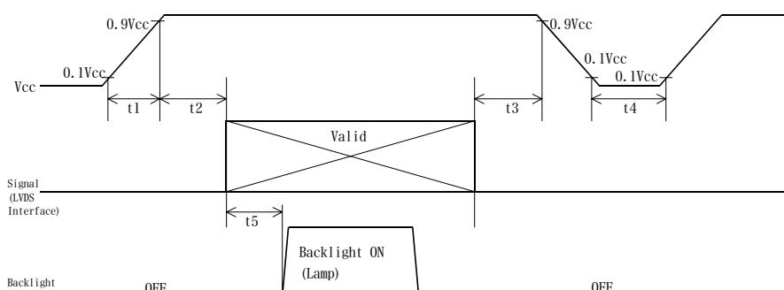
Power sequence for Backlight is not especially specified, however it is recommended to consider some timing difference between LVDS input and Backlight input as shown above.
