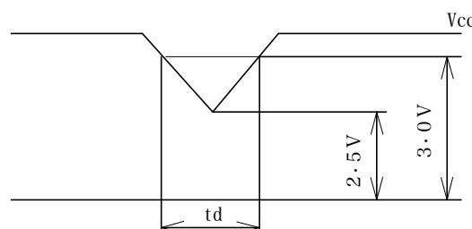
Vcc-dip conditions should also follow the On-off conditions for supply voltage .
