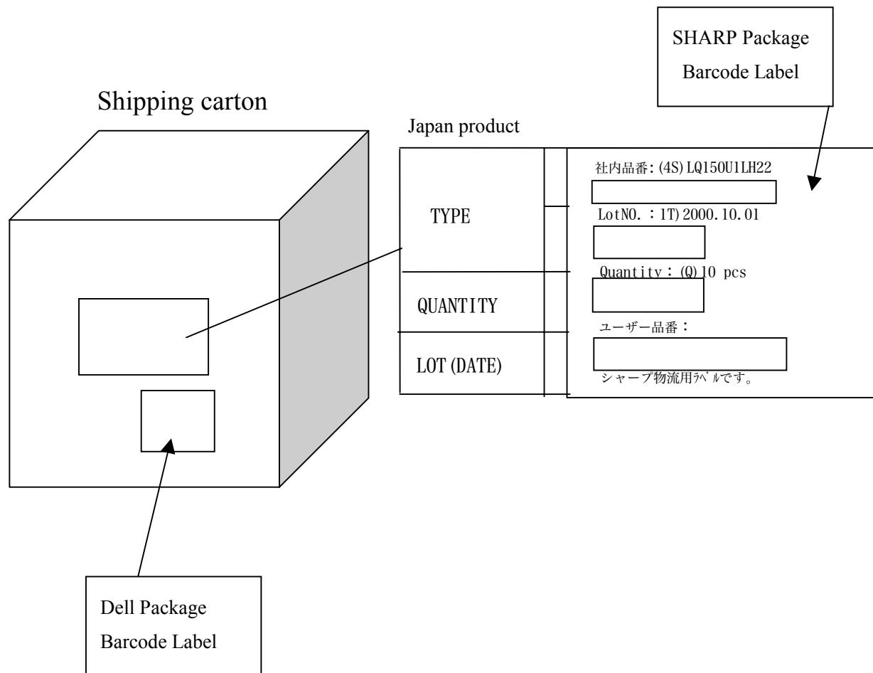
Fig3-2. Location of barcode label attachment
