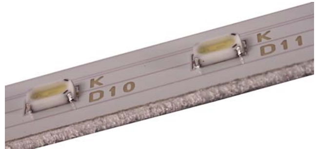
Figure 1. Closeup of LED Backlight Assembly
