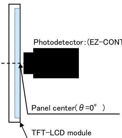
fig.2-1 Measuring method of Viewing angle range.
