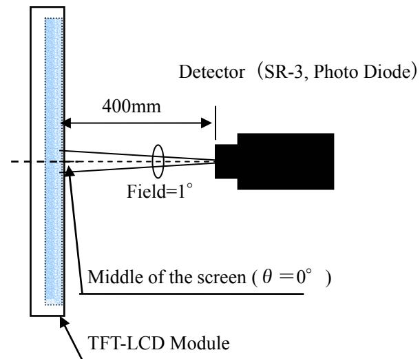
Fig.3-2 Measurement of Contrast and Luminance and chromaticity and Response time.
