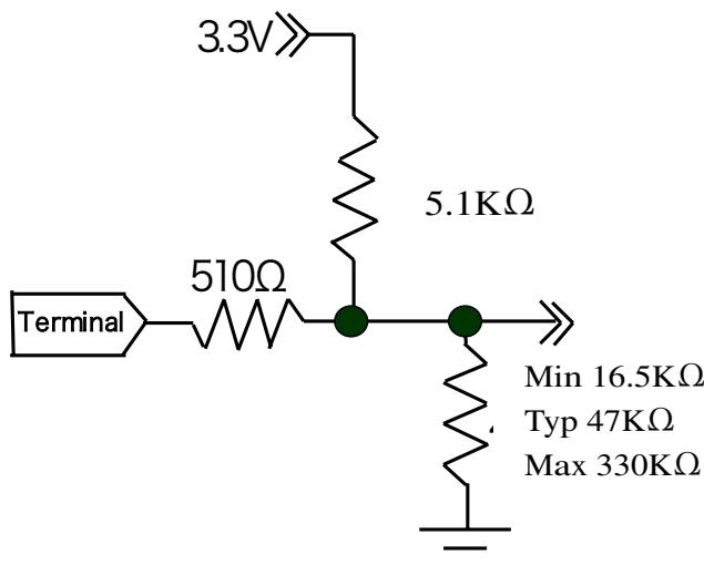
According as the surface temperature of the panel, enter the optimum 3 bit signal into pin No.4,5,6.
