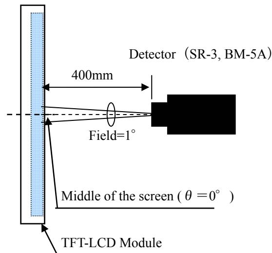
Fig.3-1 Measurement of viewing angle range.
