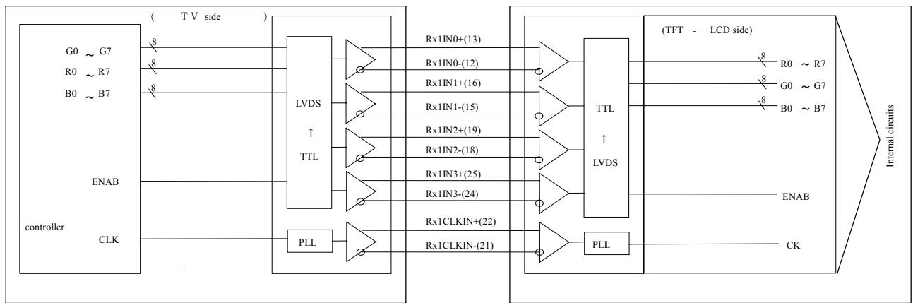
• Block Diagram (LCD Module)
