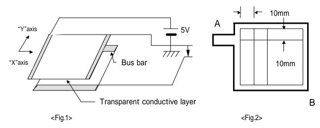
When the output voltage corresponding to every measurement position is plotted as shown in Fig.3, the difference between the voltage enclosed by the positions "A" and "B" and the output voltage at the same position shall be " Ex" (or " Ey") and the electric potential difference "EABx" (or "EABy") between "A" and "B" shall be defined as the linearity.
