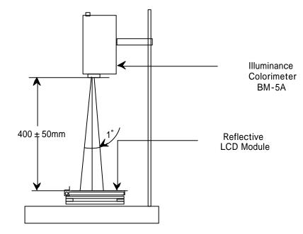
(a) The apparatus for Luminance measurement
