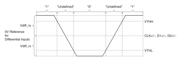
Differential Inputs Logical "0"s and "1"s, Threshold High/Low, Differential Voltage Range
