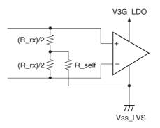
Note) 1. R\_self is used if a transmitter is not driven Clock (CLK+/–) or Data (D1+/–, D0+/–) channels.
