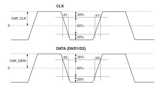
The FlatLink3G receiver is understanding that there is logical "1" when a differential voltage is more than VTHH and the FlatLink3G receiver is understanding that there is logical "0" when a differential voltage is more than VTHH. There is undefined state if the differential voltage is less than VTHH and less than VTHH. A reference figure is below.
