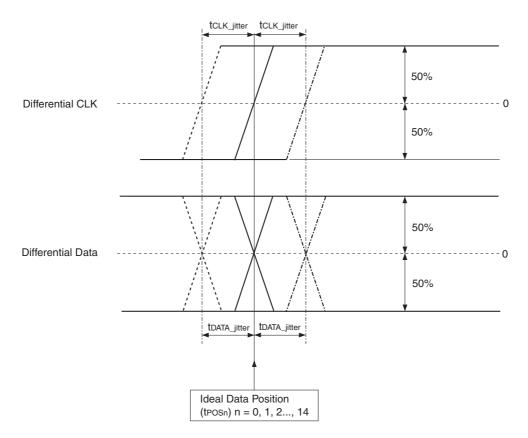
**Clock and Data Jitters - Two Data Channel Case**
