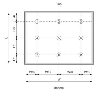
Fig. 7. The Spot Locations for Luminance Measurement
