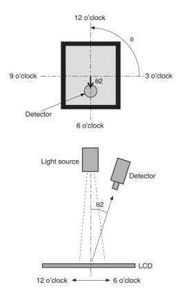
Fig. 3. Setup for Measurement C
