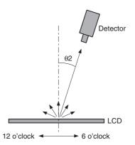
Fig. 4. Setup for Measurement D
