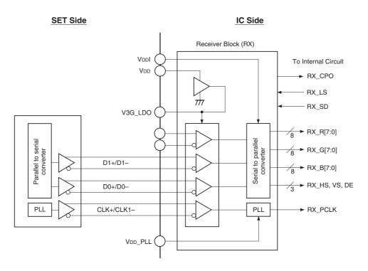
VDDI is a link power and logic level supply and GND is a ground level of all circuits from a system power supply.
