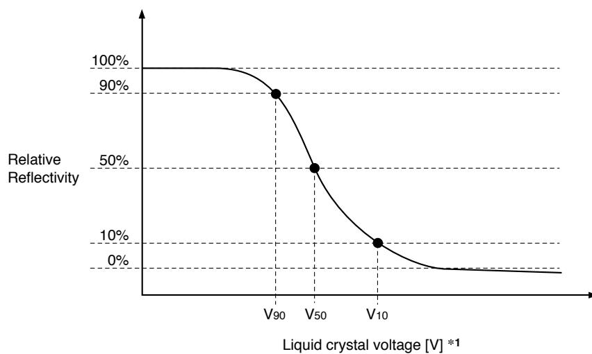
\*1 Liquid crystal voltage = I Selected voltage level – Common voltage + Reference voltage center – Common voltage center I
