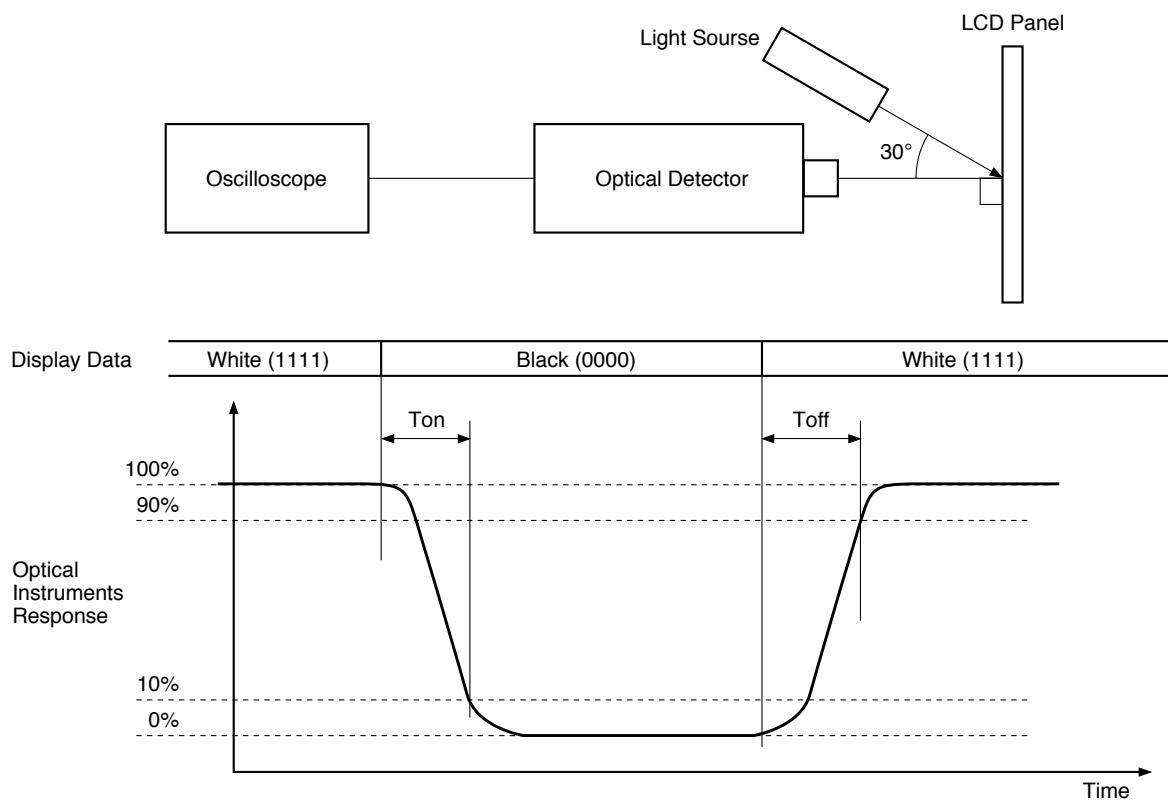
**Fig. 3. Measurement System-3**
