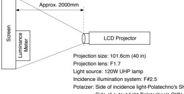
Polarzer: Side of incidence light-Polatechno's SHC-128U Side of output light-Polatechno's SKN-18243
