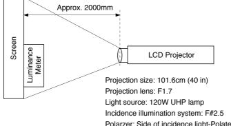
Polarzer: Side of incidence light-Polatechno's SHC-128U Side of output light-Polatechno's SKN-18243
