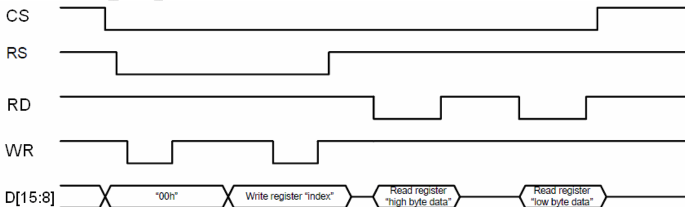
Figure 5.3.2.1 i80 8-bit System Bus Interface Timing
