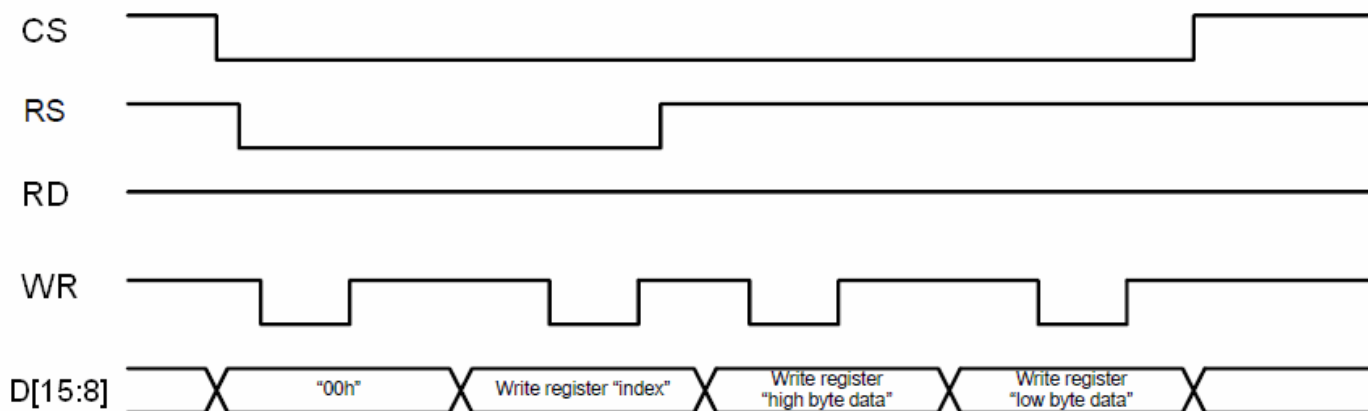
Figure 5.3.1.1 i80 8-bit System Bus Interface Timing
