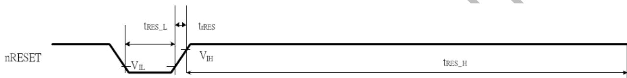
**Figure 5.2 RESET Timing**
