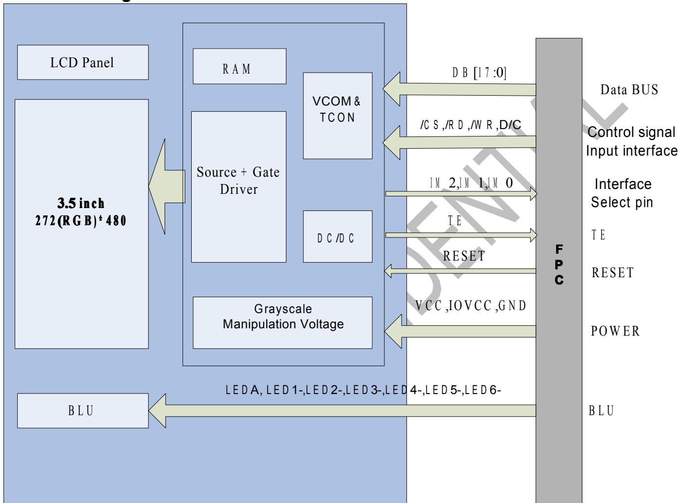
Figure 4.3 LCD module diagram
