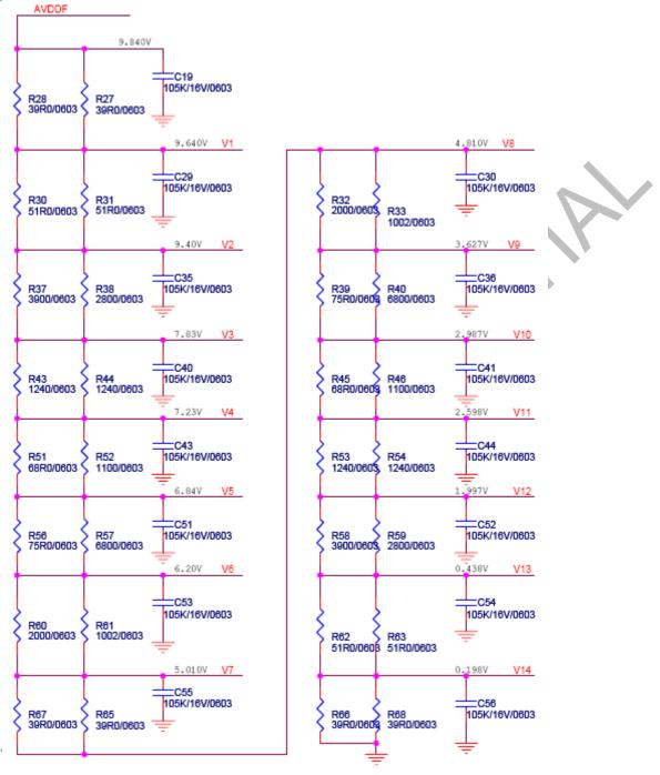
NOTE: The gamma circuit only apply to AVDD=9.840V,Connect LCM to the gamma circuit and keep LCM operation, you can get correct gamma voltage, V1=9.64V \ V2=9.40V etc.
