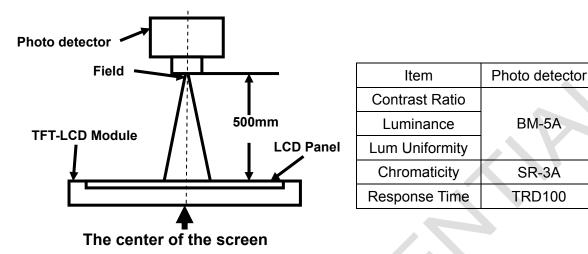
Note 2: Definition of viewing angle range and measurement system.
