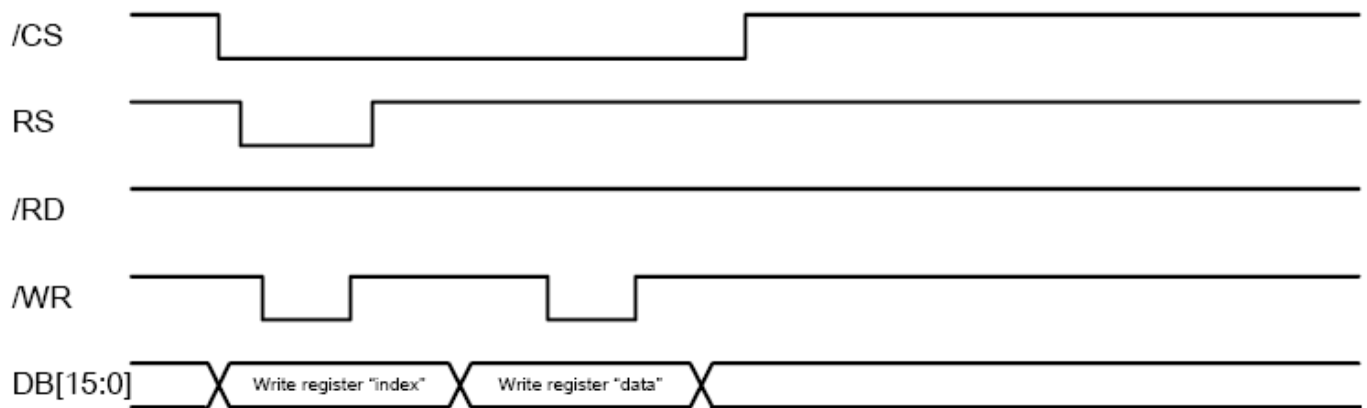
Figure 5.1.2 I80 16-bit System Bus Interface Timing
