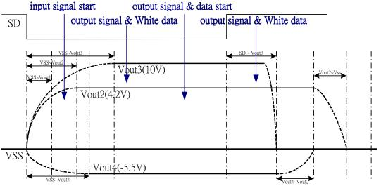
Power ON :VDD-> input signal -> 4.2V -> -5.5V -> 10V -> White data & signal output -> data output Power OFF :White data & signal output -> 10V -> -5.5V -> 4.2V -> VDD
