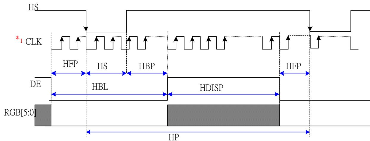
\*<sub>1</sub> The frequency of CLK should keep in the range as input timing chart determined whether in display or blanking region to ensure IC operating normally.
