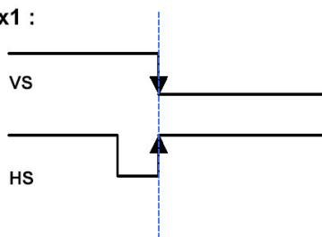
If the VS falling edge and HS rising edge are in the same time, the timing is in the margin and not surely which is the first valid data line.
