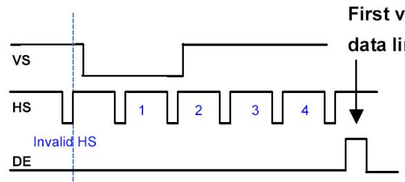
If VS falling edge is delay some time after HS rising edge, this timing will cause the first valid data line delay one HS time.
