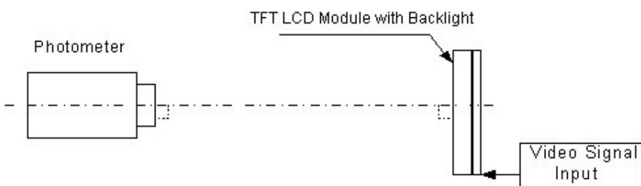
Note 9-1: Viewing angle diagrams (Measure System A)
