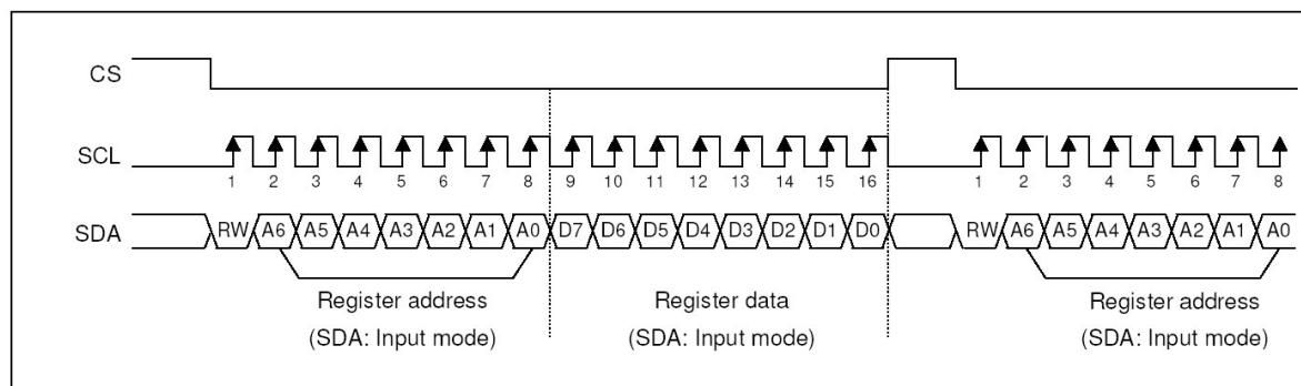
The shift register and counter are reset to their initial values when the chip select signal is inactive. Do not set the chip select signal to inactive between transmission of an 8-bit address and 8-bit data set for the command.
