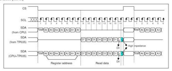
The read mode of the interface means that the micro controller reads data from the LCM.
