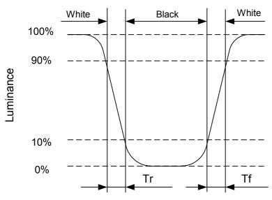
Note 9-6: Contrast Ratio in back light On (Measure System B)
