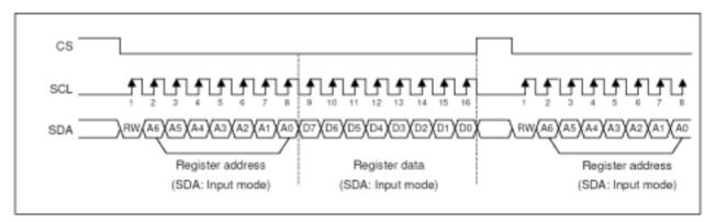
The shift register and counter are reset to their initial values when the chip select signal is inactive. Do not set the chip select signal to inactive between transmission of an 8-bit address and 8-bit data set for the command.
