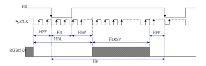
\*<sub>1.</sub> The frequency of CLK should be continued whether in display or blank region to ensure IC operating normally.
