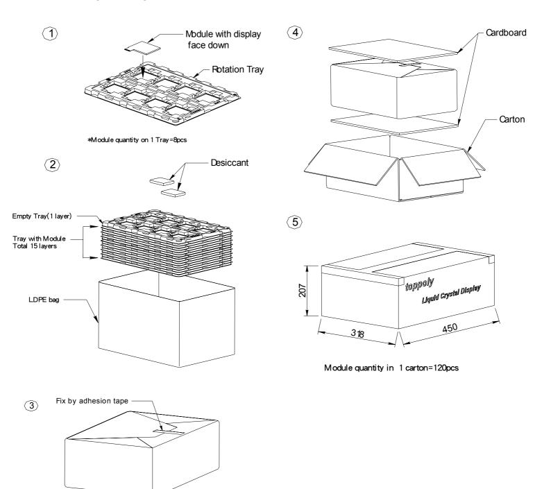
TD035SHEC1 module delivery packing method
