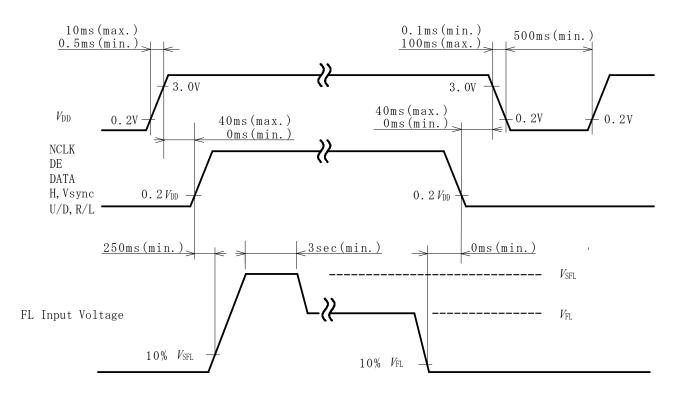
Note 1) When turn  $V_{DD}$  on and turn it off, the form of voltage should be input with not ripple signal.
