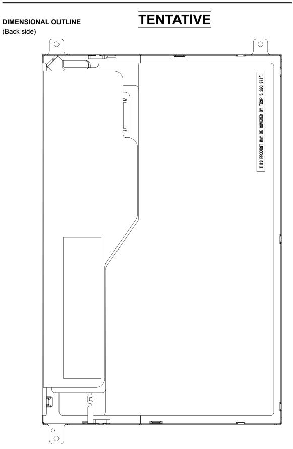
Note 1) Never push LCD back side. If LCD back side was pressed, It may cause damage of the back light system.
