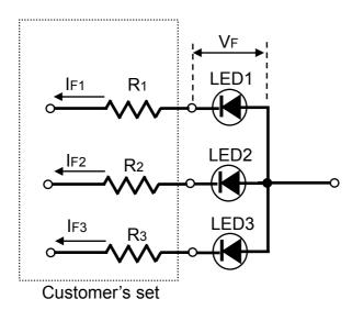
VF: Forward voltage of LED (In case of IF1, IF2, IF3=20mA: VF=3.75V)
