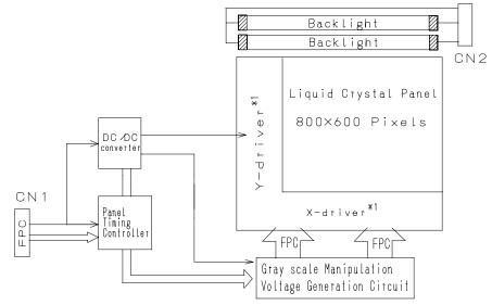
\*1 Build up LCD drivers on the glass substrate
