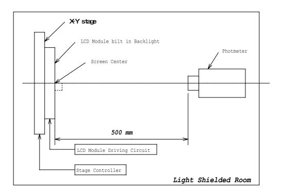
(1) The measurement point is the center of the active area except for the measurement of Luminance Uniformity.
