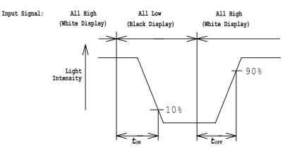
$t_{ON}$ : Turn on time is the time for a photo detector output waveform to go from maximum value to 10% of its maximum.  $t_{OFF}$ : Turn off time is the time for a photo detector output waveform to go from zero to 90% of its maximum.
