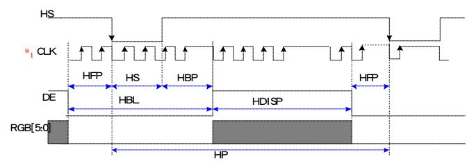
The frequency of CLK should be continued whether in display or blank region to ensure IC operating normally.
