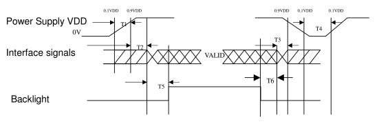
$T1 \leq 10ms \quad 0 \leq T2 \leq 50ms \quad 0 \leq T3 \leq 50ms \quad 400ms \leq T4 \quad 200ms \leq T5 \quad 100ms \leq T6$
