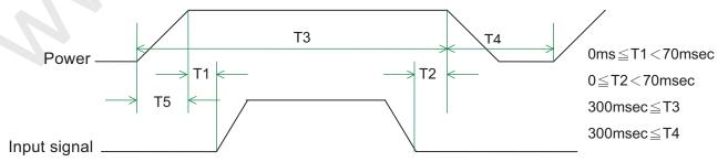
Apply the lamp voltage within the LCD operating range. When the backlight turns on before the LCD operation or the LCD turns off before the backlight turns off, the display may momentally become abnormal.
